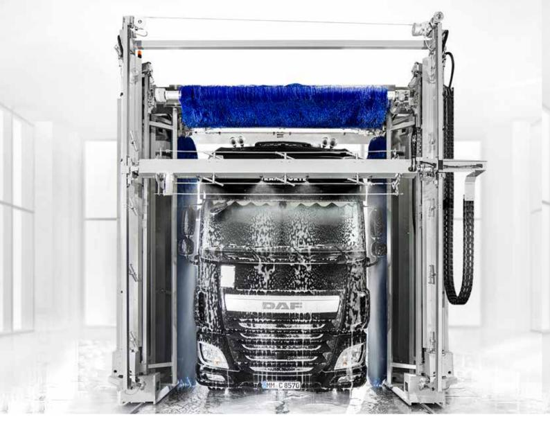
Pre-spray device with chemistry integrated in the horizontal beam JETSTREAM
